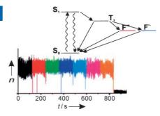
On the ROXS: Photobleaching represents one of the main limitations of modern fluorescence microscopy. A reducing and oxidizing system (ROXS) has been introduced that recovers triplet states as well as charge-separated states through electron-transfer reactions (see picture). Thus the blinking and photobleaching of fluorophores is strikingly reduced.
