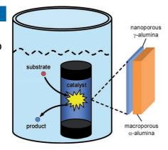
A cat with nine lives: Catalyst separation and recycling is the bane of homogeneous catalysis. This problem is addressed by a two-layered ceramic membrane cylinder that allows the diffusion of reactants and products in and out, but keeps the catalyst trapped. The concept is demonstrated for the enantioselective transfer hydrogenation of acetophenone to (S)-phenylethyl alcohol with large molecular catalysts anchored on Fréchet-type dendrimers.
